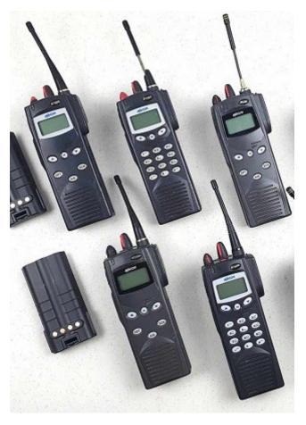
The M7100 and P7100 look almost identical to the M7200 and P7200. Check the label to confirm the model number. The M7200 and P7200 are 700 MHz capable and can remain fully functional on the DTR system.
