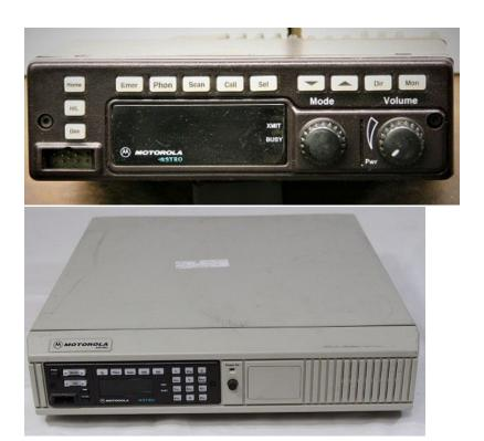
Some XTL5000 models have similar looking control heads to the Astro Spectra, so check the model label on the radio body to confirm whether the unit is an Astro Spectra or an XTL5000. The XTL5000 supports 700 MHz and can remain fully functional on the DTR system. If "XTL5000" is not visible on the label, the unit is an Astro Spectra or Astro Spectra Plus. The XTL5000 units will display "XTL5000" while booting, while the Astro Spectra will display "SELF CHK" or "SPECTRA+".
